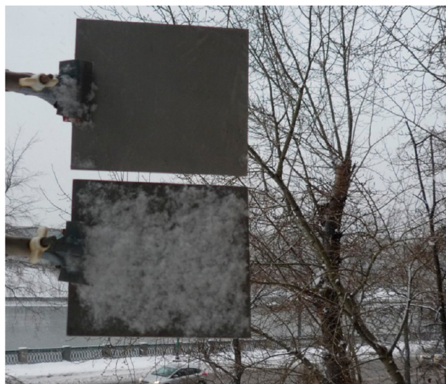
Figure 3. Outdoor test of comparative behavior of sample 3 with a superhydrophobic coating (top) and untreated stainless steel (bottom) in heavy snowfall at -3\text{ }^{\circ}\text{C} , relative humidity 99%, and wind velocity 2\text{ m s}^{-1} .
